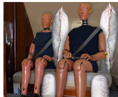
Side facing inflatable solutions for passengers occupying a divan.
